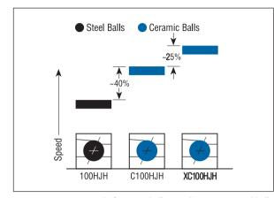
Running speed of ceramic ball exceed same-size steel ball by 40%. Converting to an X-Life Ultra Bearing with ceramic balls will boost running speeds an additional 25%.
