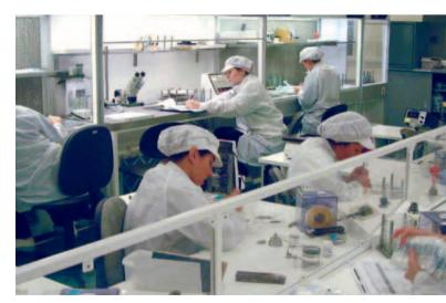
All Barden precision bearings are assembled under stringent cleanroom conditions.
