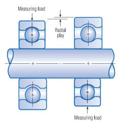
Fig. 3. Radial play is a measure of internal clearance and is influenced by measuring load and installation practices. A high radial play value is not an indication of lower quality or less precision.
