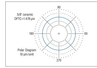
Deviation from true circularity (DFTC). Polar trace of a 5/8" silicon nitride ball indicates near perfect roundness, which results in dramatically lower vibration levels.
