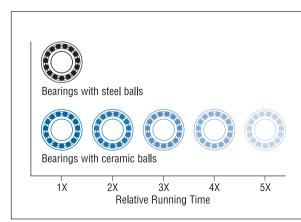
Service life of ceramic hybrid bearings is two to five times that of conventional steel ball bearings, depending upon operating conditions.
