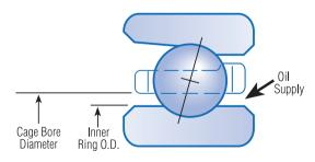
**■ Fig. 17.** Lubrication window for B-type bearings.
