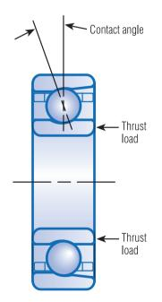
**Fig. 4.** Contact angle refers to the nominal angle between the ball-to-race contact line and a plane through the ball centers, perpendicular to the bearing axis.
