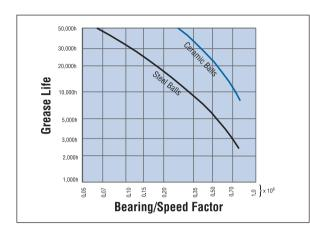
The use of ceramic balls significantly increases bearing grease life performance.
