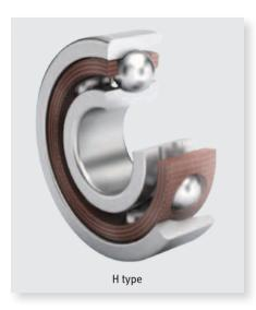
Non-Separable Type (H): Inner ring has full shoulders, outer has one shoulder cut away with a small retaining lip at the edge of the raceway.
