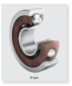
**Separable Type (B):** Outer ring has full shoulders, inner ring has one shoulder cut away. The inner ring is removable for mounting on the shaft separately from the outer ring assembly.
