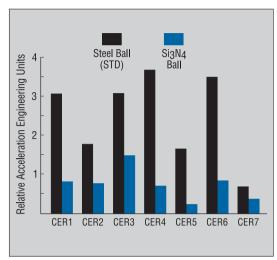
Vibration tests comparing spindles with steel ball bearings and the same spindle retrofit with ceramic hybrids.
